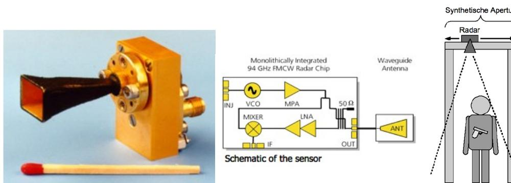
**Figure 9: Miniturized 94 GHz FM-CW Radar module and block diagram of the sensor. The right picture shows the principle of the SAR-system.**
