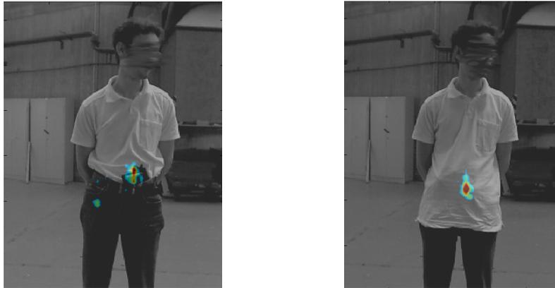
**Figure 10: SAR measurement at 94GHz. The optical image is superposed by the radar image. This gives a good impression, where hidden objects can be found. Size and shape of the objects cannot be seen so easily.**
