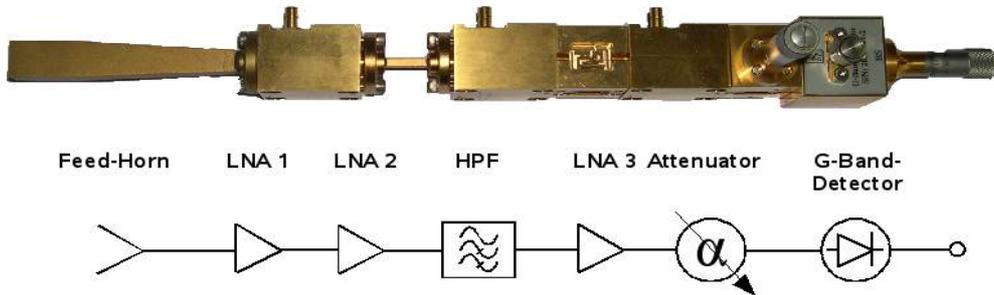
Figure 2: Photograph of the 220 GHz front-end. From left to right: Receiving horn, first LNA stage, second LNA stage, high-pass filter, third LNA stage, attenuator and detector.
