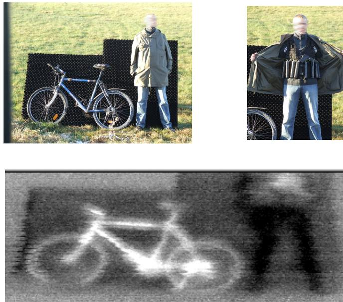
**Figure 7: Radiometric image at 220 GHz showing a bicycle and a person wearing a bomb vest underneath the jacket. Person and bicycle were standing in front of absorber material to increase the contrast. The radiometric image on the left represents raw data, on the right side the image after post-processing is shown.**
