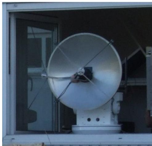
**Figure 1: Radiometric System for standoff detection of concealed weapons working at 220 GHz.**
