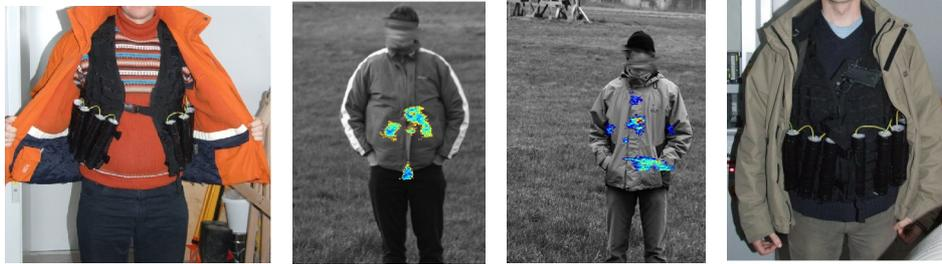
**Figure 6: Optical image of scanned persons. The prominent parts of the radiometric images have been superimposed on the images. In the left picture the bomb vest worn beneath the jacket can clearly be seen. Additionally, you can see the belt-buckle. On the right image the hidden gun can be clearly identified together with some metallic object hidden in the right pocket.**
