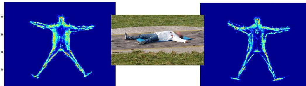
**Figure 11: Typical ISAR measurements of a person lying down on the turntable. The measurement distance was 135 m at a frequency of 220 GHz and 8GHz bandwidth. Measurement time was 2 minutes. In the left picture the person was wearing a bomb vest. The tubes filled with metal can easily be recognized.**
