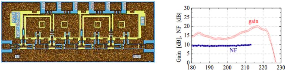
Figure 3: Left: Chip photograph of a four-stage 220 GHz cascode low-noise amplifier MMIC. The chip-size is 1x2.5mm<sup>2</sup>. Right: Measured gain and noise figure (NF) of a 220 GHz low-noise amplifier module.
