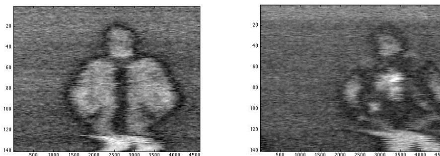
**Figure 5: Scan of a person. Left: Without weapon. Right: With hidden weapon. The gun worn at the chest can be clearly identified.**
