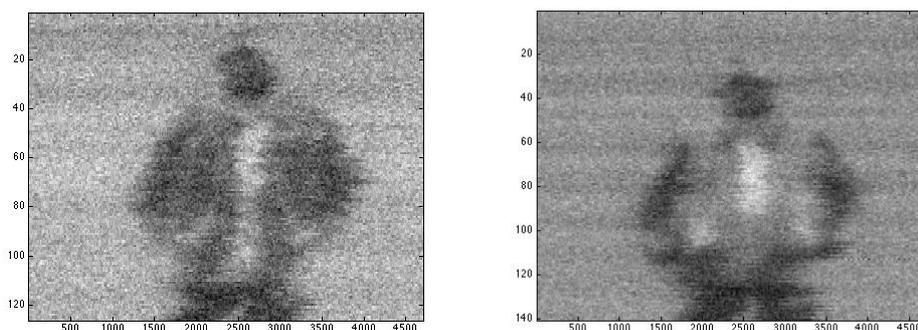
**Figure 4: Scan of a person at 10 m distance. Left: Without bomb vest or weapon. Right: Person wearing a bomb vest under the coat.**
